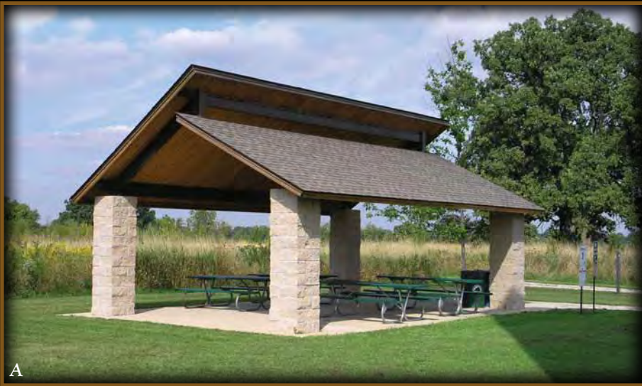
Forest Preserve, Batavia, IL: 20' x 30' Northwest model with 2" x 6" T & G sub-roof and fascia with shingles. Stone surrounds by others.
