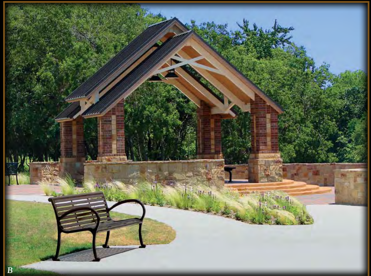
Markwood Park, Irving, TX: 20' x 20' Aspen model with 12" o.c. Weathered Copper color standing seam steel roof with a 2" x 6" T & G sub-roof. Stone and brick by others.
